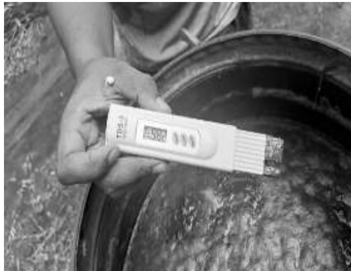
Figure 13. Measurement of TDS (Total Dissolved Solids) value in one of the cow's breeders organic fertilizer in Lau Damak Village
